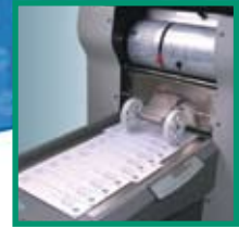
Automatic extending conveyor activated by the number of forms processed
